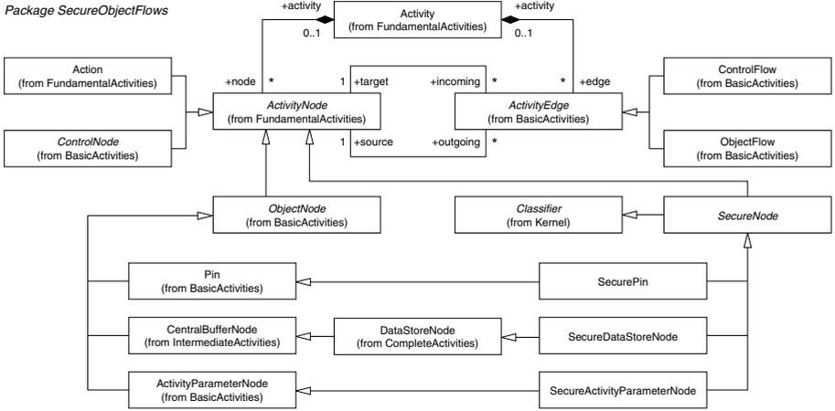
**Fig. 1.** UML metamodel extension for secure object flows
