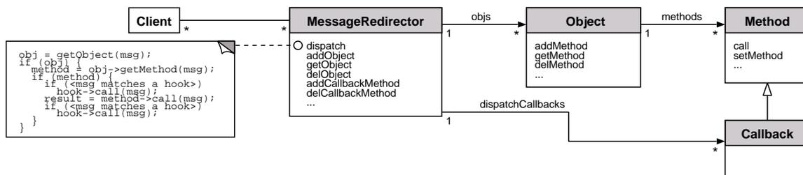
Figure 3. Class-Based Design of a MESSAGE REDIRECTOR
