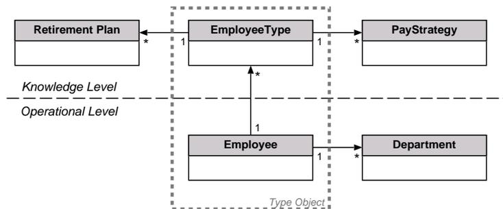
Figure 1. Employee Type Knowledge Level Using a Type Object
